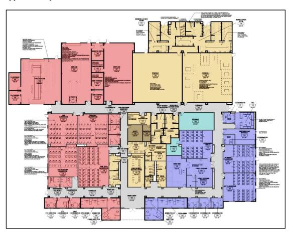
The apparatus building is designed for the storage of the programs' multiple fire training vehicles including fire trucks, emergency medical and rapid response vehicles, and HAZ MAT trailers. The building is equipped with modern vehicle exhaust extraction systems to provide a safe environment. Other areas include secure storage for the multiple disciplines and an office.
